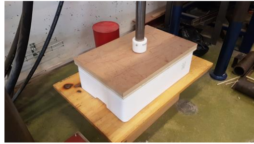
Figure 2. 15-kg box under uniformly distributed vertical top load.
