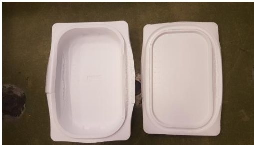
Figure 1. Broken 3-kg box (left) and lid (right) after having been loaded with around 510 kg weight on top of the box with lid on.
