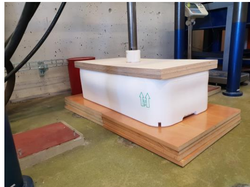
Figure 3. New 23-kg box with drain holes under uniformly distributed vertical top load.
